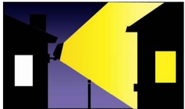
Full-cut-off fixture (permitted) vs. Outdoor luminaire that creates light trespass (prohibited)
