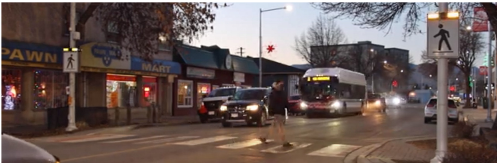
Crosswalk with Rectangular Rapid Flashing Beacon on Tranquille Road (see policy 27)
