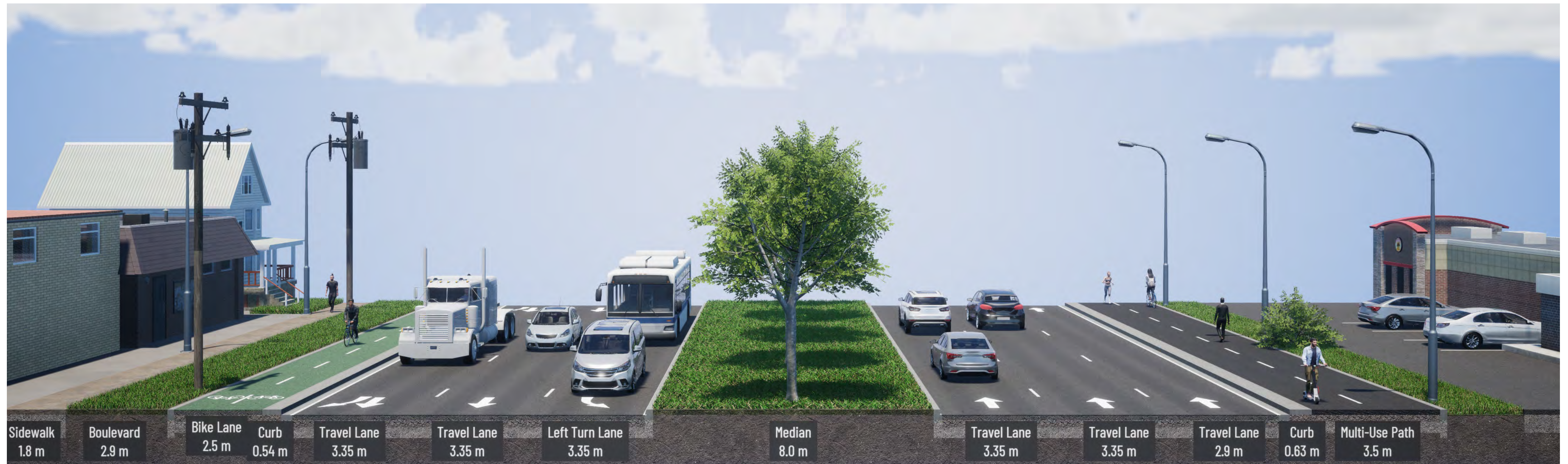
Sample cross section of two-way protected bike lanes on Provencher Boulevard facing east
