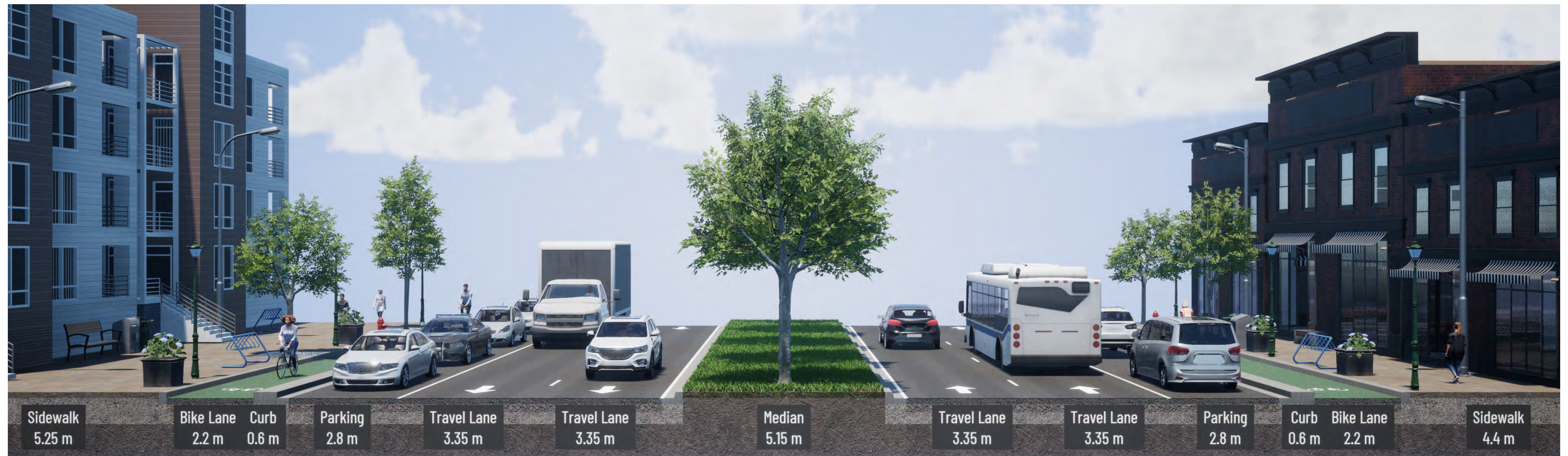
Sample cross section of one-way protected bike lanes on Provencher Boulevard facing east
