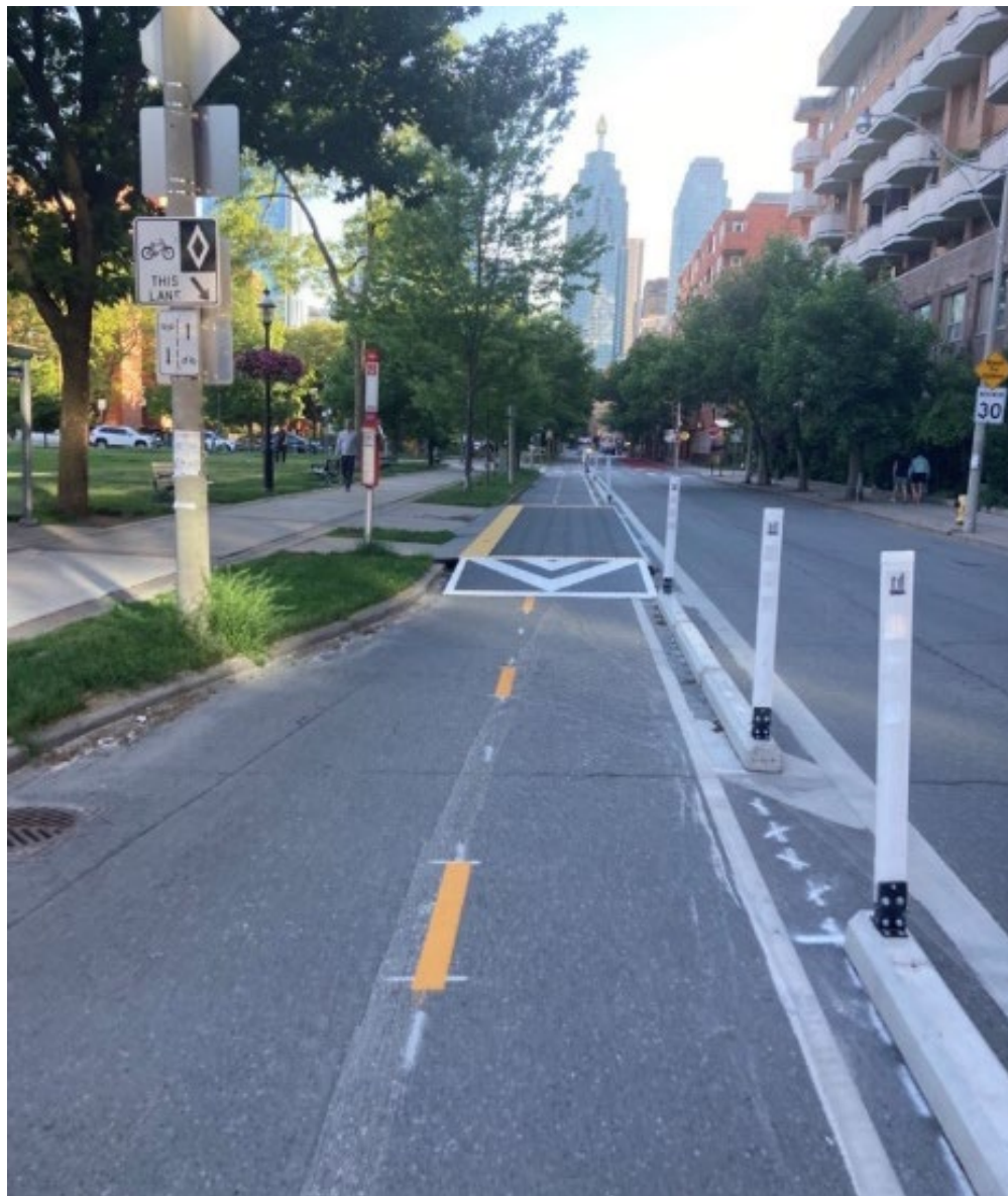
Figure 3.3: Retrofit Bidirectional Physically Separated Bicycle Lane
