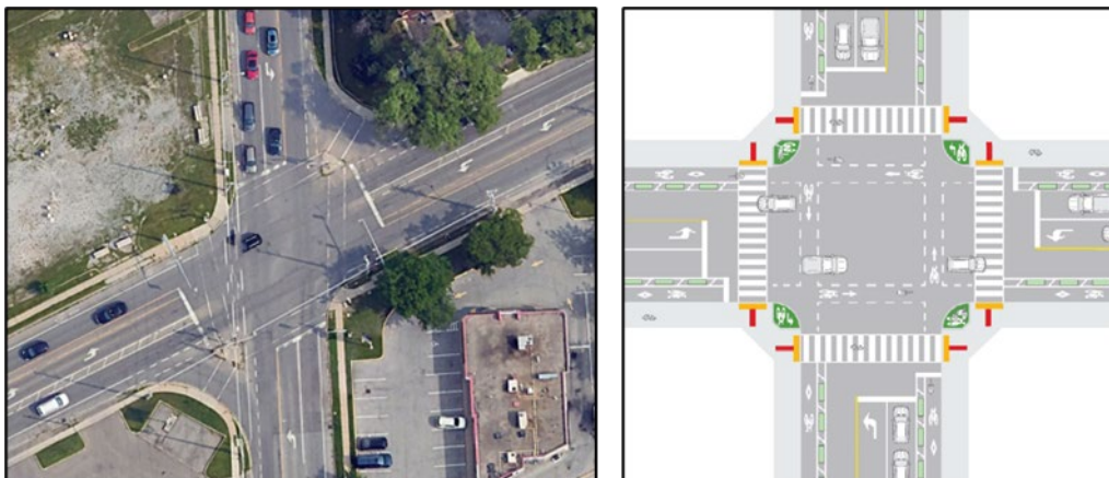
Figure 2.3 – (Left) Existing intersection at Scott Street and Vine Street. (Right) Protected intersection for cyclist identified in OTM Book 18.
