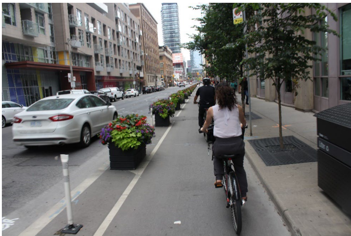
Figure 5.3: One-Way Separated Bicycle Lane With Planters, Toronto
