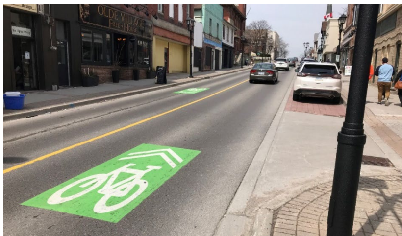
Figure 5.11: Narrow Shared Lane with Sharrows, Newmarket
