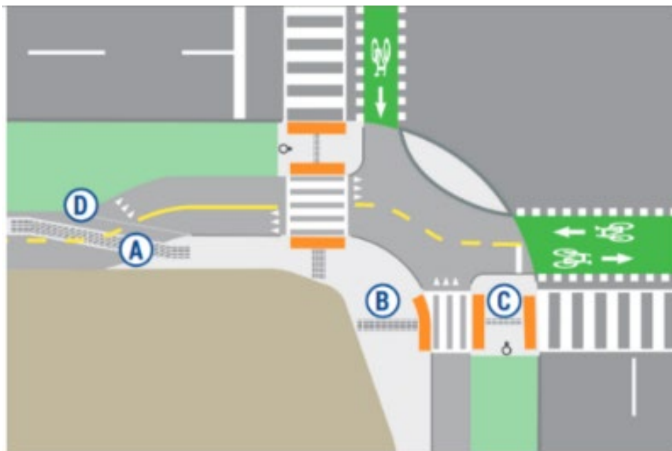
Figure 6.2. Standard protected corner showing directional TWSI at transition from MUP to separated facilities where pedestrians have the straight path of travel (preferred)
