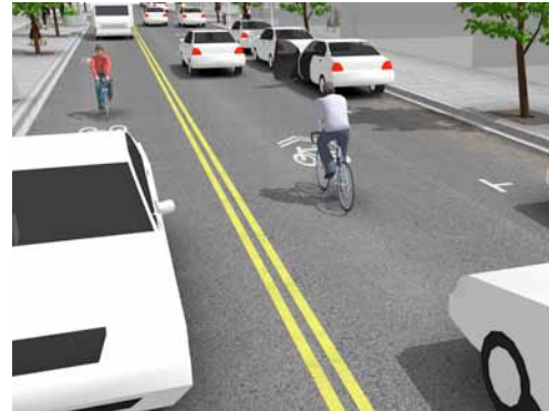
Confident cyclists may share the vehicle lane Source: NACTO Urban Bikeway Design Guideline
