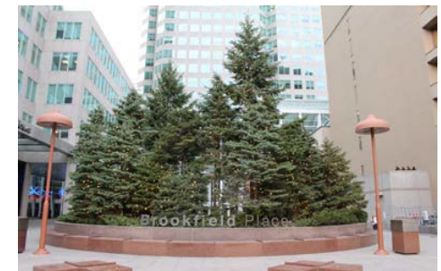
Image 12: Examples of wind control measures for winds between buildings
